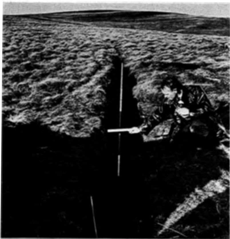
Fig. 3. Mining subsidence fissure at ground surface.
